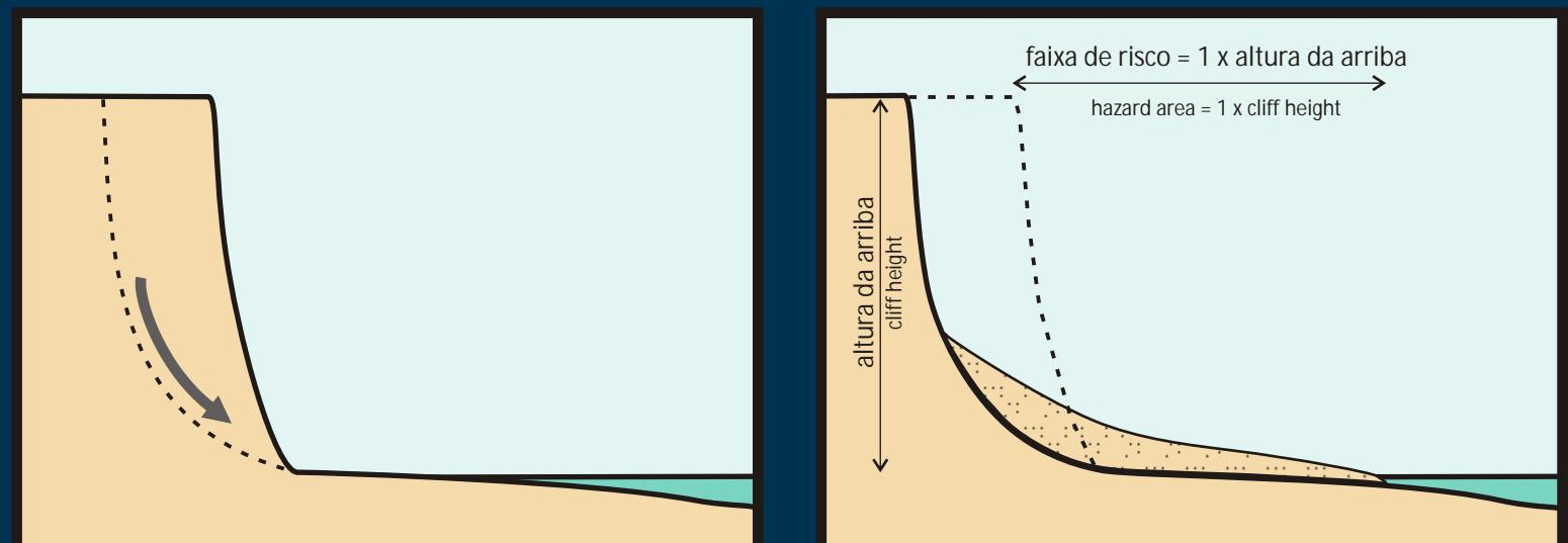
Natural cliff evolution (erosion) progresses by intermittent and discontinuous series of cliff collapses. Cliff evolution is a potential menace for people standing on beaches accumulated at the cliff base. HAZARD AREAS correspond to areas where it is likely that effects of debris will be felt and its length equals 1 time cliff height. For your safety, keep away from cliff base and cliff edge.
